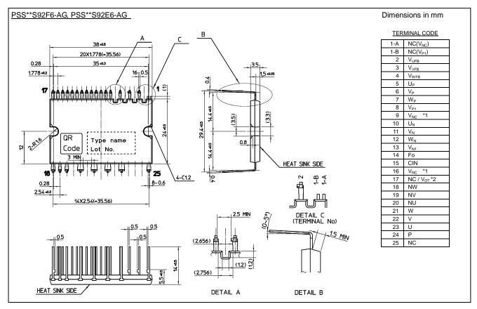
1) 9 & 16 pins (V<sub>NC</sub>) are connected inside DIPIPM, please connect either one to the control power supply GND outside and leave another one open.
