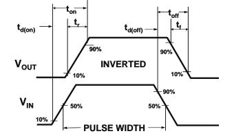
Figure 2:Switching Waveforms
