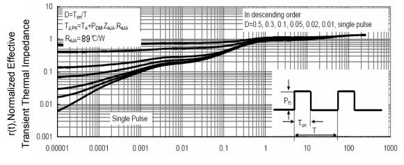
Square Wave Pluse Duration(sec) Figure 13 Normalized Maximum Transient Thermal Impedance
