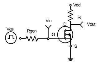
Figure 1:Switching Test Circuit
