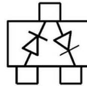
MMBD4148 Marking:5H    MMBD4148CA Marking:D6    MMBD4148CC Marking:D5    MMBD4148SE Marking:D4
