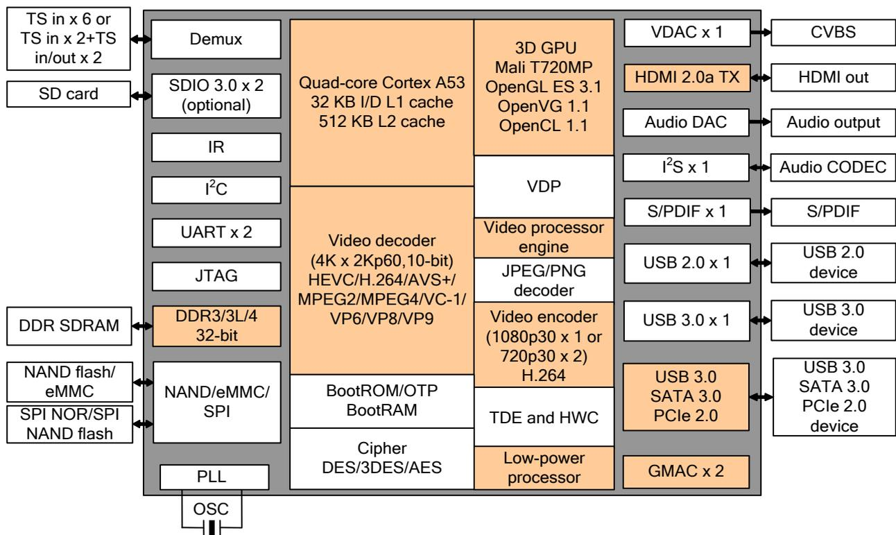
Hi3798C V200 is an ultra-HD high performance SoC supporting 4Kp60 fps decoding for the DVB and IPTV STB markets. With an integrated quad-core 64-bit high-performance Cortex A53 processor and embedded NEON, Hi3798C V200 provides powerful CPU
