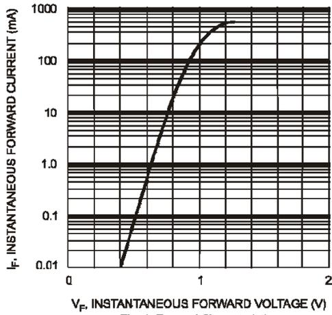
Fig. 1 Forward Characteristics
