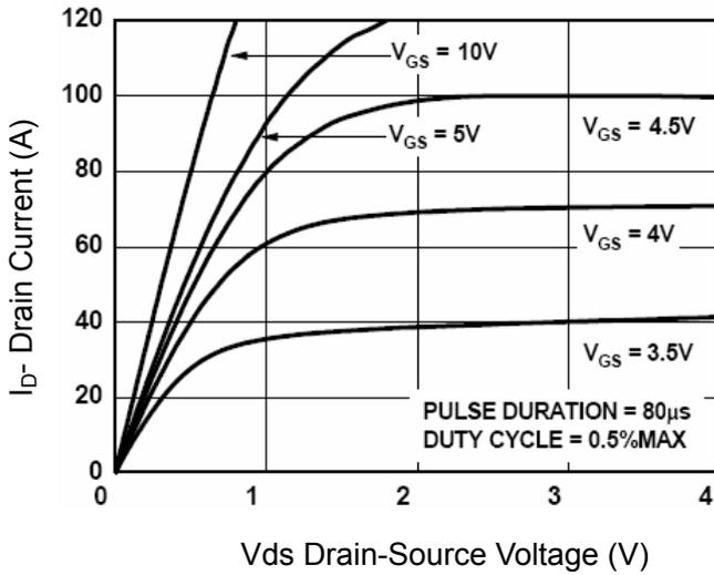
Figure 1 Output Characteristics
