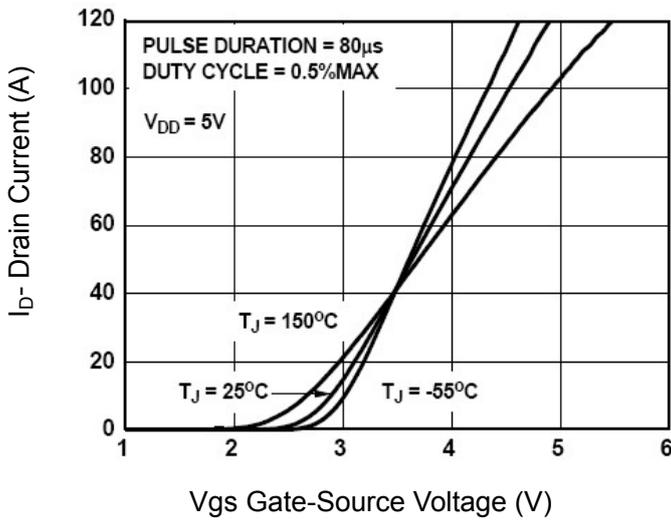
Figure 2 Transfer Characteristics
