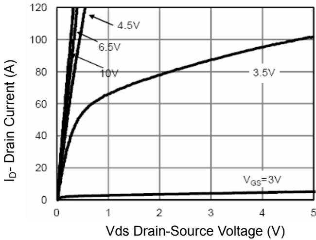
Figure 1 Output Characteristics
