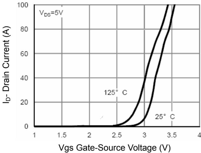
Figure 2 Transfer Characteristics
