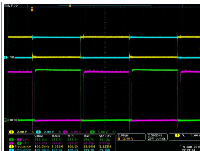
图 42. Bench Test Waveform for INA/B and OUTA/B
