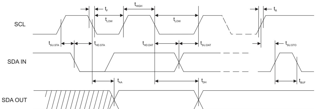
**Figure 6-3. Write Cycle Timing**
