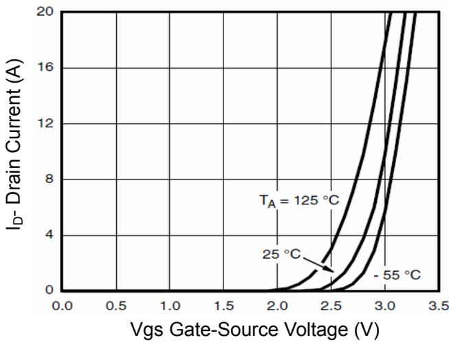
Figure 2 Transfer Characteristics
