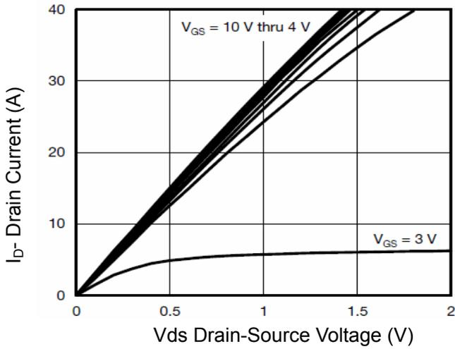
Figure 1 Output Characteristics
