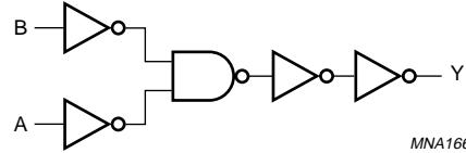
Fig.4 Logic diagram.
