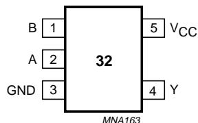
Fig.1 Pin configuration.
