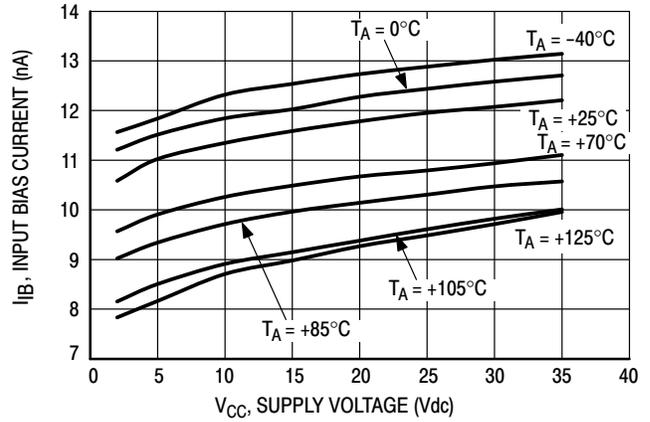
Figure 3. Input Bias Current versus Power Supply Voltage
