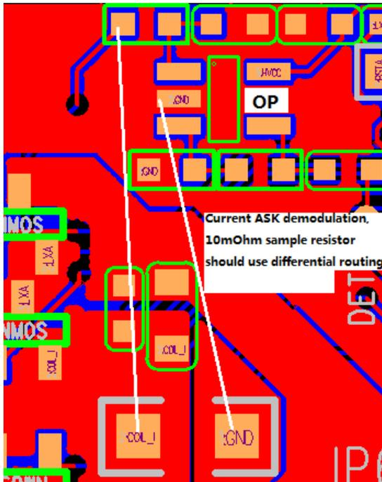
3. CODE\_DET\_I and CODE\_DET\_V are sensitive signals should be wrapped up by ground and placed far away from switching MOSFET.
