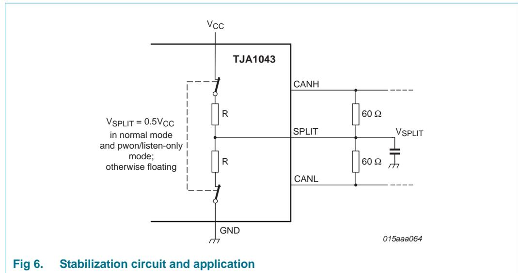
**Fig 6. Stabilization circuit and application**
