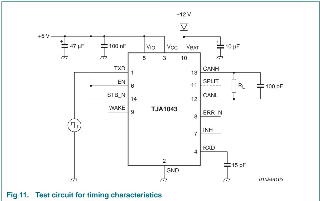
Fig 11. Test circuit for timing characteristics
