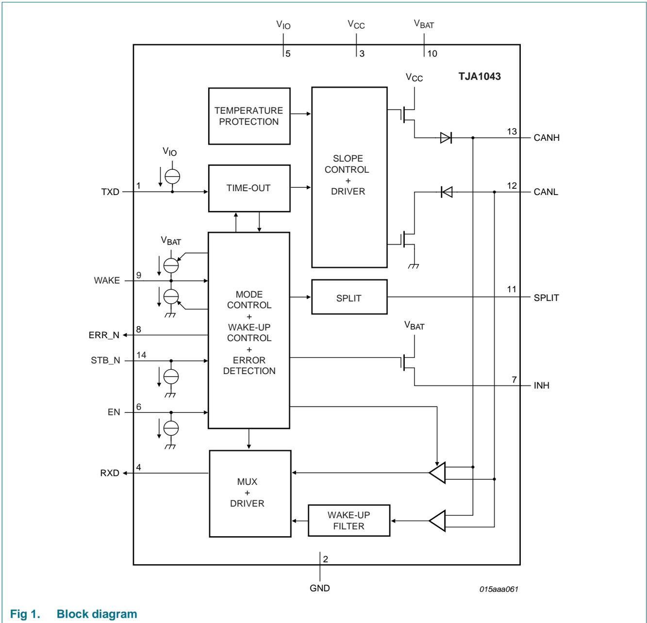
Fig 1. Block diagram
