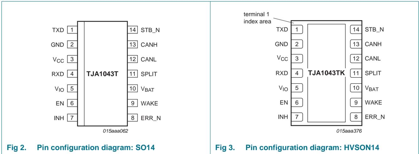
Fig 2. Pin configuration diagram: SO14
