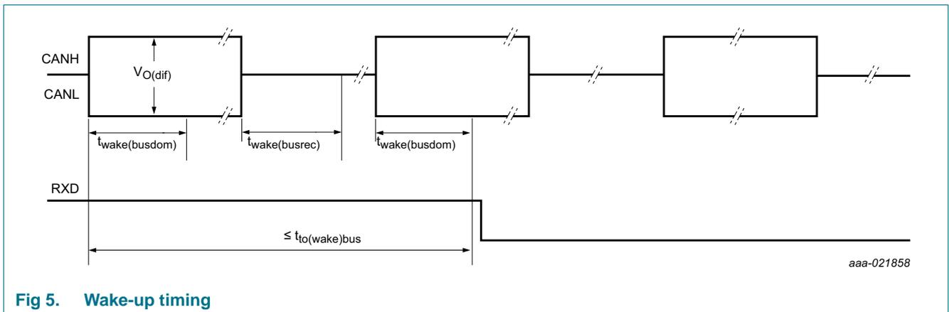
Fig 5. Wake-up timing
