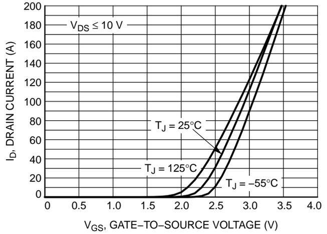
Figure 2. Transfer Characteristics
