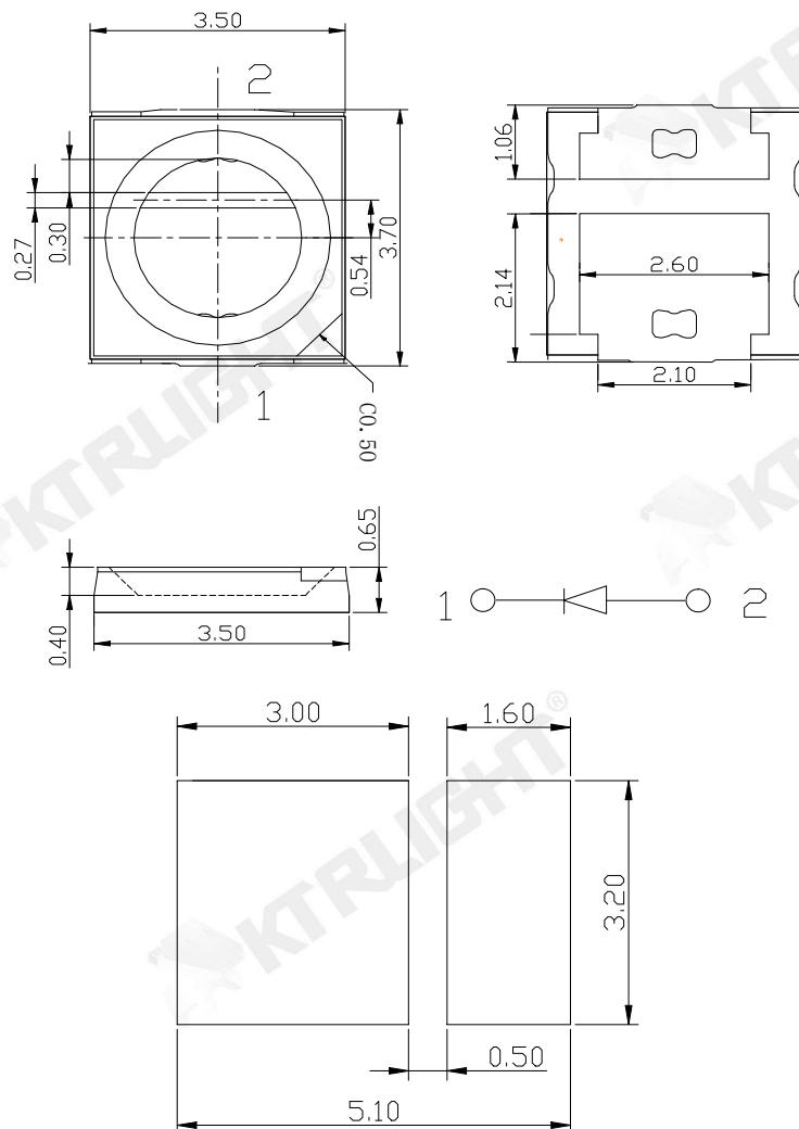
推荐焊盘式样(Recommended Soldering Patter )
