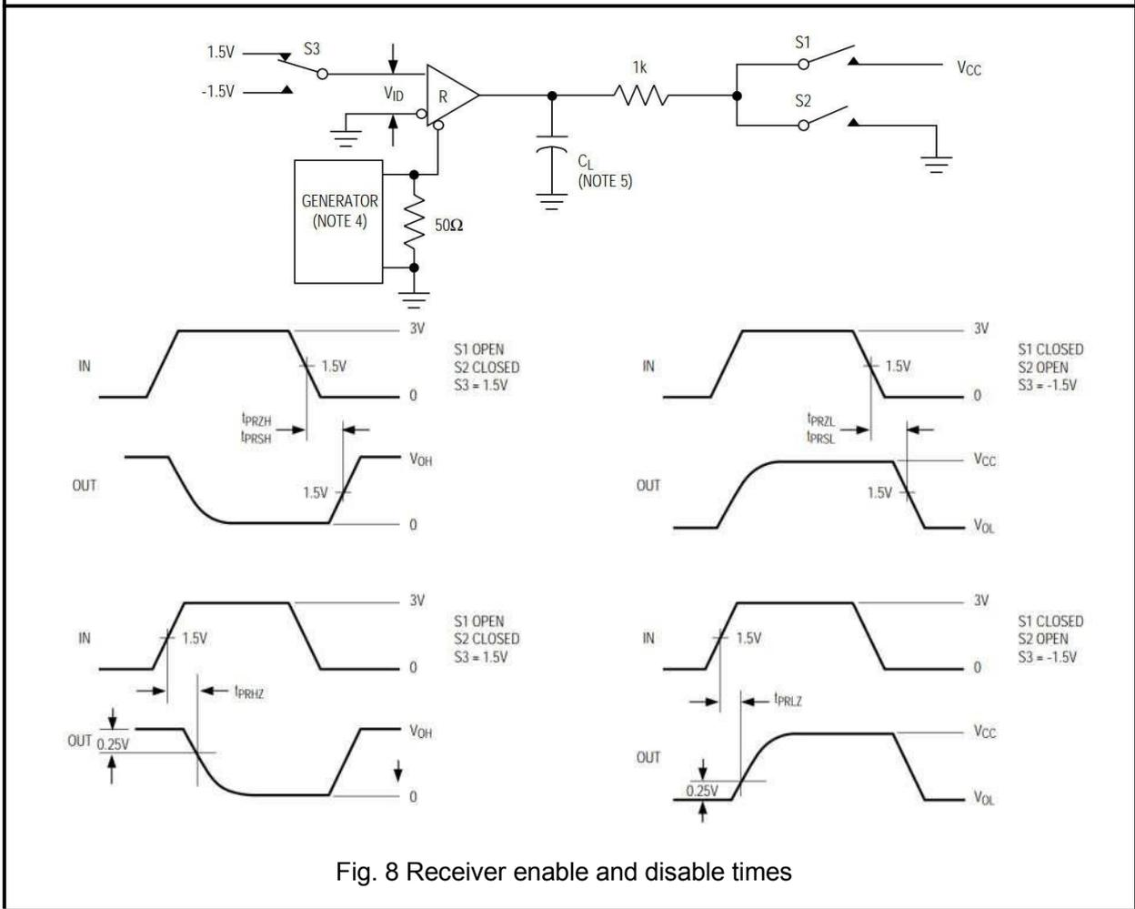
Fig. 8 Receiver enable and disable times
