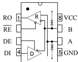
Figure 1 MAX3485E pin configuration
