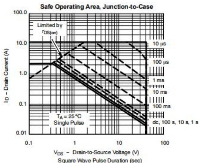
TYPICAL ELECTRICAL AND THERMAL CHARACTERISTICS
