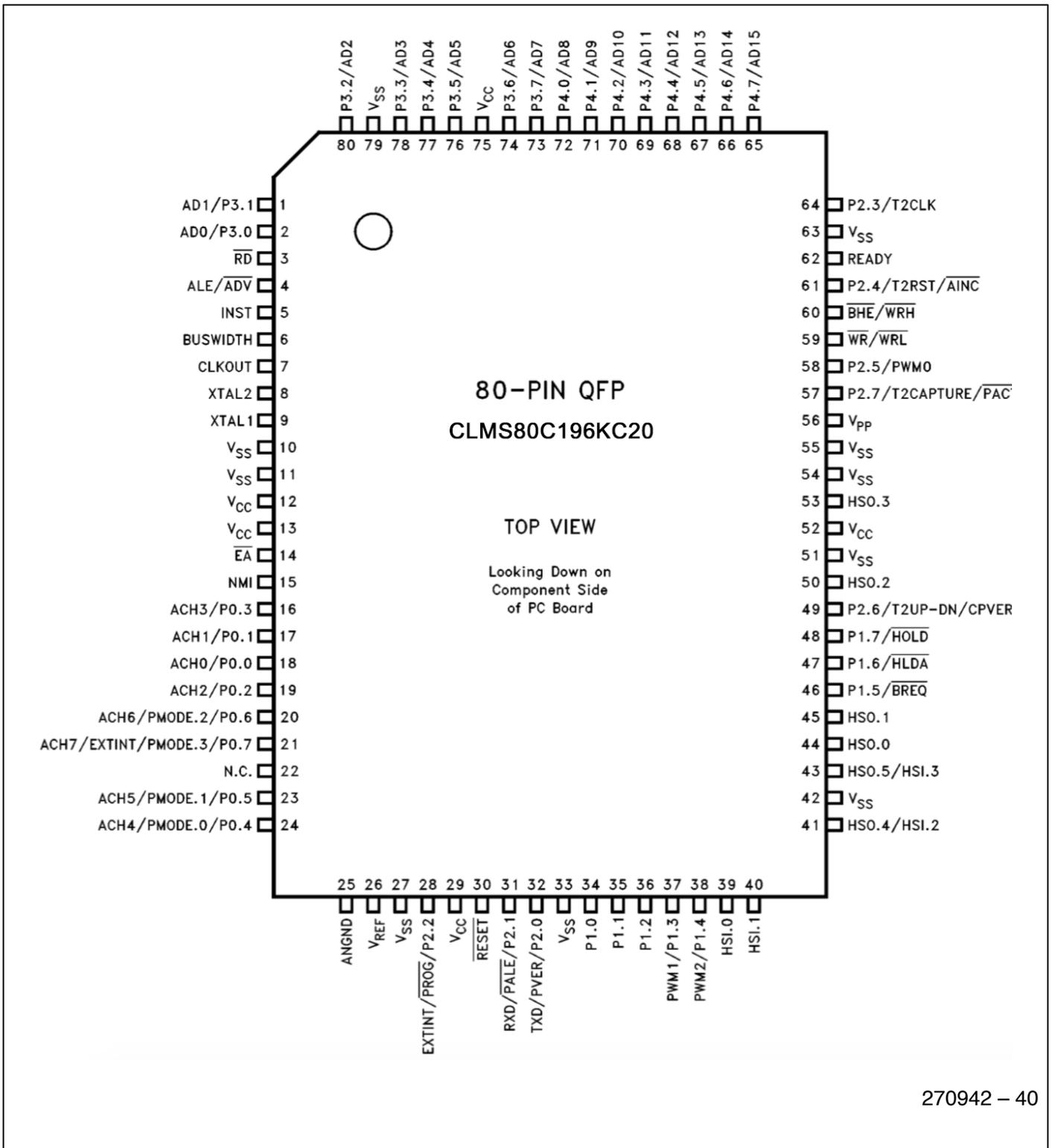
图5. S80C196KC20 80-Pin QFP封装
