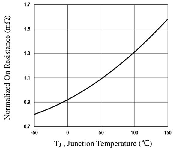
**Fig.2 Normalized R<sub>DS(on)</sub> vs.  $T_J$**
