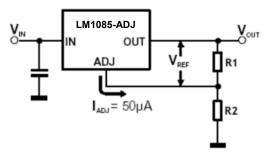
The LM1085 series develops a 1.25V reference voltage between the output and the adjust terminal. Placing a resistor between these two terminals causes a constant current to flow through R1 and down through R2 to set the overall output voltage.
