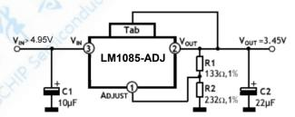
$$V_{OUT} = V_{REF} \times ~(1 + \frac{R2}{R1}) ~ + I_{ADJ} \times R2 \label{eq:VOUT}$$
