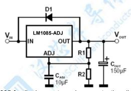
Unlike older regulators, the LM1085 family does not need any protection diodes between the adjustment pin and the output and from the output to the input to prevent over-stressing the die.
