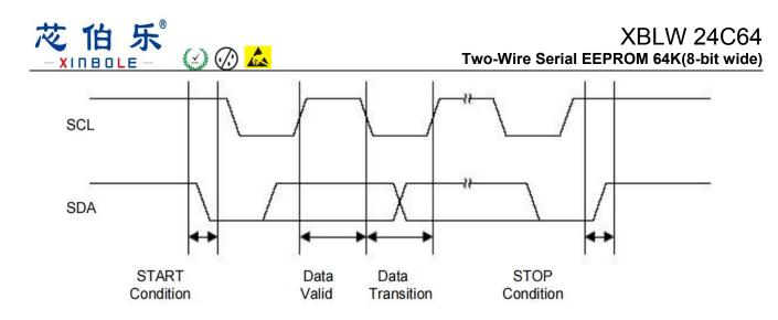
Figure1: Timing diagram for START and STOP conditions
