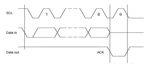
Figure 2: Timing diagram for output ACKNOWLEDGE
