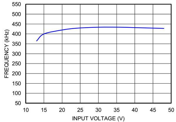
图 8-3. Frequency versus Input Voltage ( $I_{OUT} = 100 mA$ )
