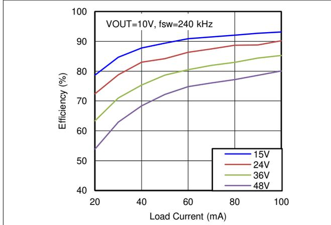
图 6-1. Efficiency at 240 kHz, 10 V
