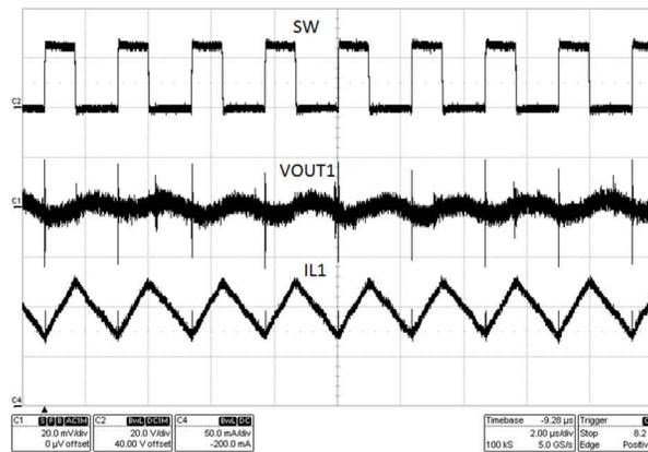
图 8-4. Typical Switching Waveform ( $V_{IN} = 24 V$ ,  $I_{OUT} = 100 mA$ )
