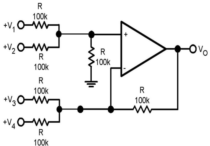
Where:  $V_0 = V_1 + V_2 - V_3 - V_4$ ,  $(V_1 + V_2) \geq (V_3 + V_4)$  to keep  $V_0 > 0$  VDC
