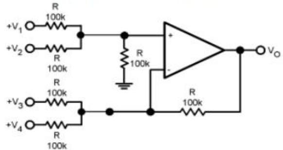
Where:  $V_O = V_1 + V_2 - V_3 - V_4$ , ( $V_1 + V_2 \geq V_3 + V_4$ ) to keep  $V_O \geq 0$   $V_{DC}$
