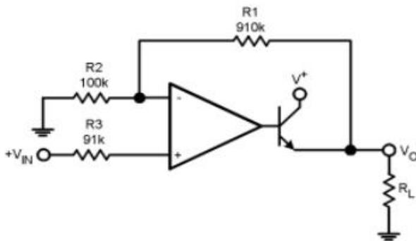
$V_O = 0$   $V_{DC}$  for  $V_{IN} = 0$   $V_{DC}$ ,  $A_V = 10$
