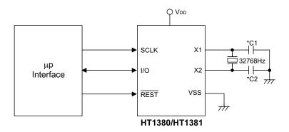
\*Note: The value of the capacity depends on how accurate the crystal is. Refer to the suggestion table of page 7.
