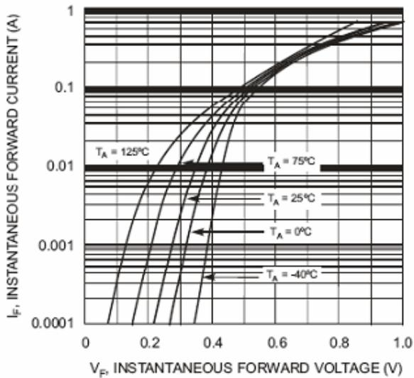
Fig. 1 Forward Characteristics
