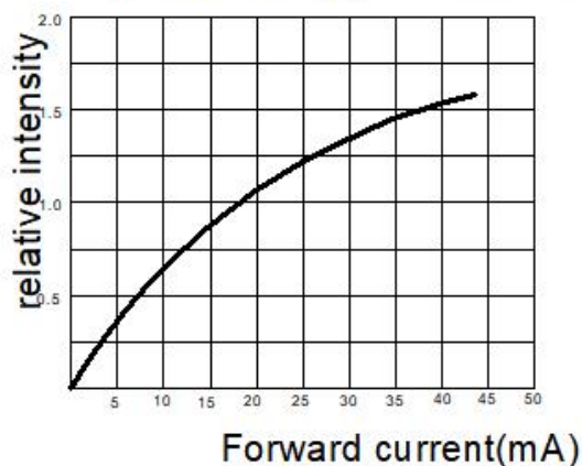
Relative light intensity vs current
