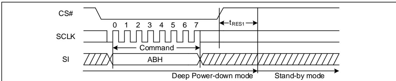
**Figure 34. Release Power-Down/Read Device ID Sequence Diagram**
