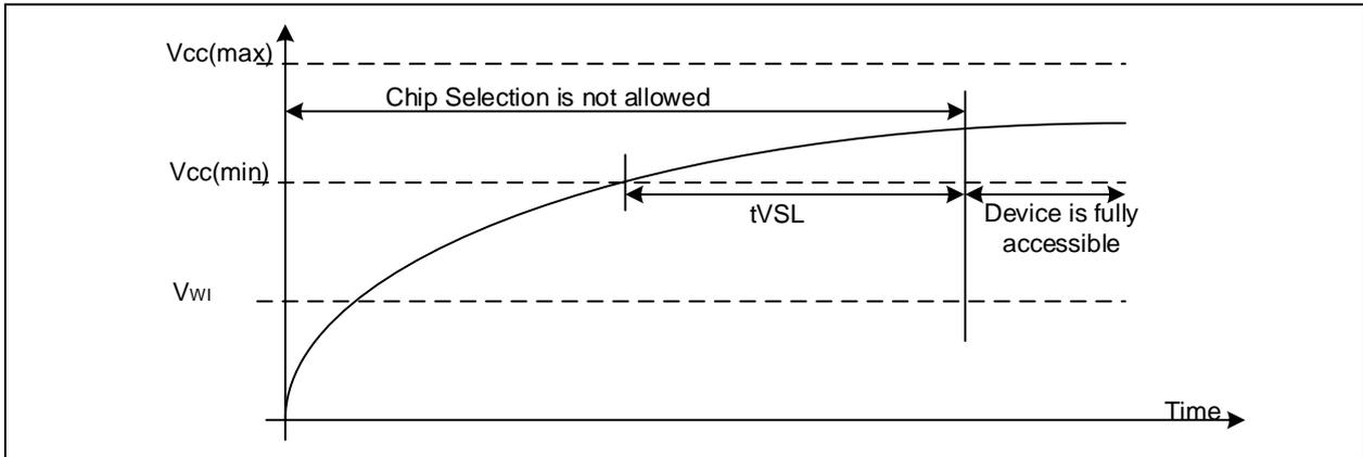
Table 12. Power-Up Timing and Write Inhibit Threshold
