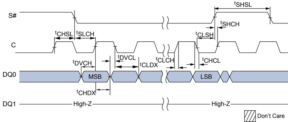
**Figure 53: Write Protect Setup and Hold During WRITE STATUS REGISTER Operation (SRWD = 1)**
