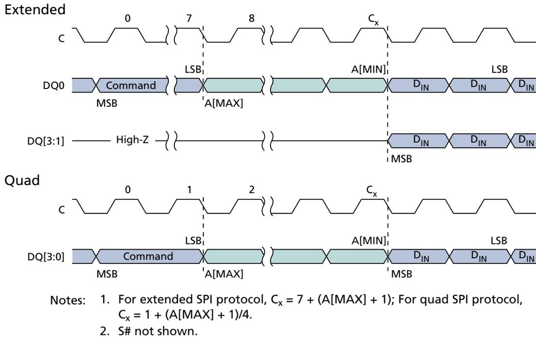
**Figure 38: EXTENDED QUAD INPUT FAST PROGRAM Command**
