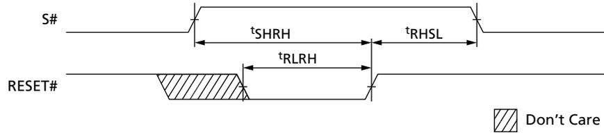
**Figure 50: Reset Enable and Reset Memory Timing**
