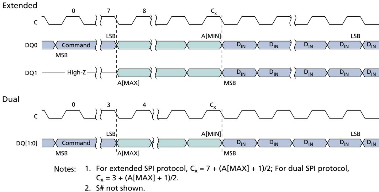
**Figure 37: QUAD INPUT FAST PROGRAM Command**
