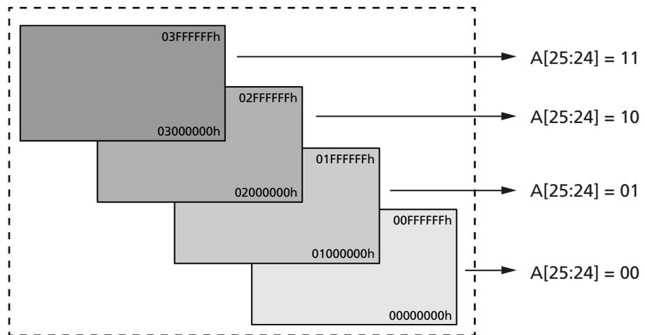
The PROGRAM and ERASE operations act upon the 128Mb segment selected in the extended address register. The BULK ERASE operation erases the entire device.
